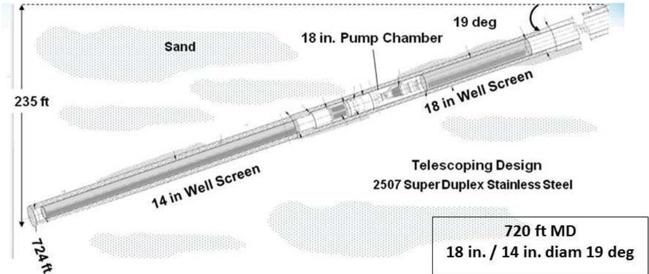
Figure 5. MPWSP Test Slant Well Showing Telescoping Design
