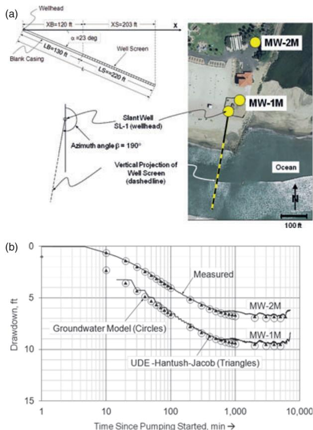
**Figure 7.** Dana Point slant well location and orientation (a). (b) Measured, modeled and UDE-calculated drawdowns for MW-1M and MW-2M ( $\alpha=23^\circ$ ,  $\beta=190^\circ$ ,  $L = 350$  ft,  $LS = 220$  ft,  $K = 426$  gpd/ft<sup>2</sup>,  $S_s = 5.85 \times 10^{-6}$ /ft,  $b = 200$  ft,  $K'/b' = 0.003$ /d,  $Q = 1660$  gpm,  $ns = 4$ ).
