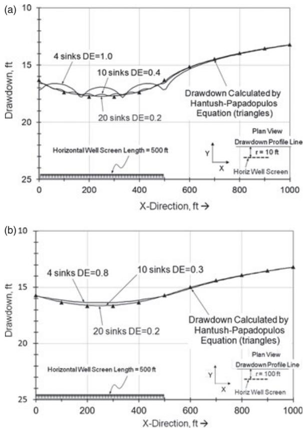
**Figure 4. Comparison of UDE drawdown profiles, (ft) for a horizontal well with the Hantush-Papadopoulos equation (a) profile 10 ft away and parallel to well, (b) 100 ft away.  $\alpha = 0^\circ$ ,  $\beta = 90^\circ$ ,  $L = LS=500$  ft,  $K = 500$  gpd/ft<sup>2</sup>,  $S_s = 1 \times 10^{-6}$ /ft,  $b = 200$  ft,  $Q = 1000$  gpm,  $t = 365$  d.**
