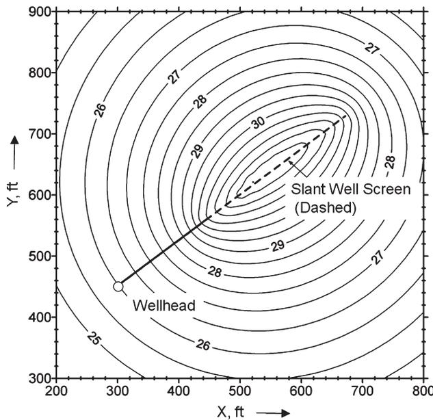
**Figure 3. Drawdown distribution (ft) in the vicinity of a slant well calculated using Equation 6.  $\alpha = 23^\circ$ ,  $\beta = 53^\circ$ ,  $L = 500$  ft,  $LS = 300$  ft,  $K = 500$  gpd/ft<sup>2</sup>,  $S_s = 1 \times 10^{-6}$ /ft,  $b = 117$  ft,  $Q = 1000$  gpm,  $t = 365$  d,  $ns = 10$ ,  $XW = 300$  ft,  $YW = 450$  ft.**
