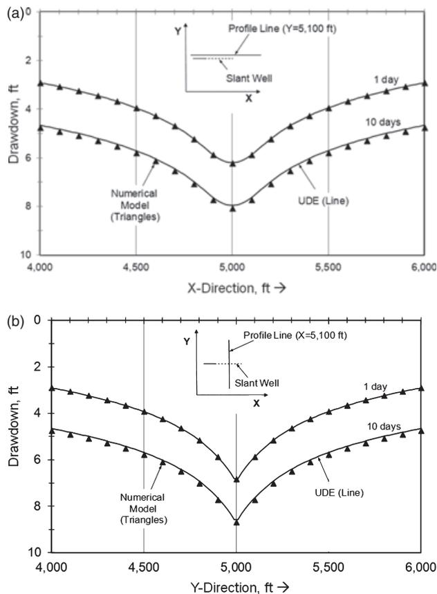
**Figure 5. Comparison of UDE (Equation 6) drawdowns in the vicinity of a slant well with numerical model drawdowns. (a) Drawdown profile is parallel to the slant well axis and (b) profile is perpendicular to the axis ( $\alpha = 45^\circ$ ,  $\beta = 90^\circ$ ,  $L = 383$  ft,  $LS = 283$  ft,  $K = 750$  gpd/ft<sup>2</sup>,  $S_s = 5 \times 10^{-6}$ /ft,  $b = 200$  ft,  $Q = 1000$  gpm,  $XW = 4829$  ft,  $YW = 5000$  ft).**
