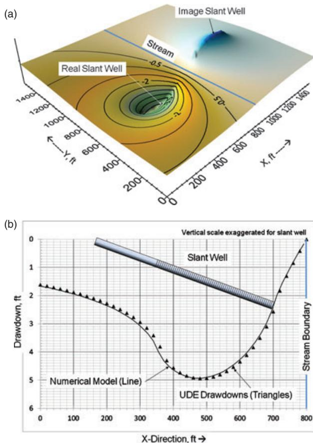
**Figure 6.** Slant well drawdowns near a stream. (a) Real and image well drawdowns using the UDE (Equation 6). (b) Cross section through  $Y = 610$  ft comparing UDE drawdowns to numerical model drawdowns. ( $\alpha = 30^\circ$ ,  $\beta = 90^\circ$ ,  $L = 500$  ft,  $LS = 400$  ft,  $K = 500$  gpd/ft<sup>2</sup>,  $S_s = 1 \times 10^{-6}$ /ft,  $b = 200$  ft,  $Q = 1000$  gpm,  $t = 10$  d,  $ns = 10$ ).
